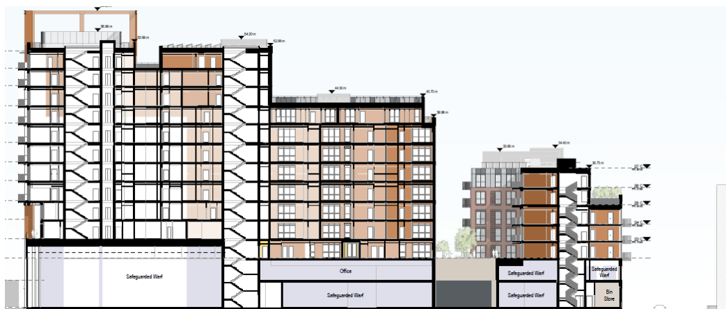
Image 13: Cross Section Wharf Box with residential above
